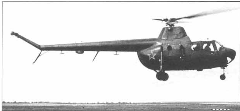
Ми-1МРК на испытаниях, 1960 г. Mi-1MPK reconnaissance and fire adjusting helicopter, 1960
